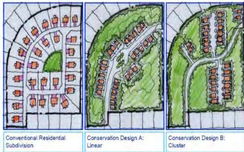
Alternative designs A and B preserve large areas of open space and reduce road construction, while providing the same number of housing units (Vision Plan drawing)
